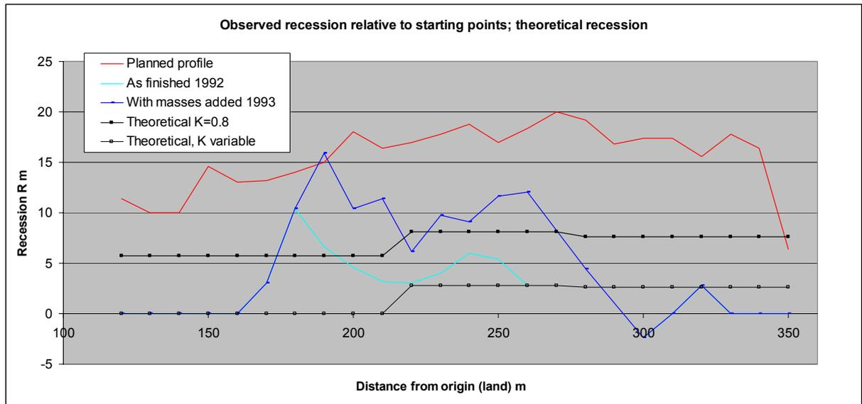
Figure 4 Observed and theoretically calculated recession. The observed recession is shown relative to different starting points, as planned (red), final profile in January 1992 (blue), and final as-built profile in August 1993 (turquoise).
