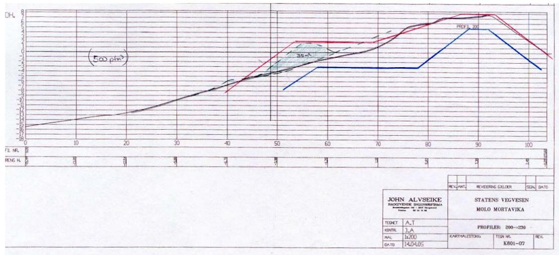
Figure 3 Result from the 2005 survey (sample). Intended profile (shown in red line), limit of primary berm layer (blue), 2005 survey (solid grey), August 2003 survey (dotted green), and volume added in 1993 (green shaded).
