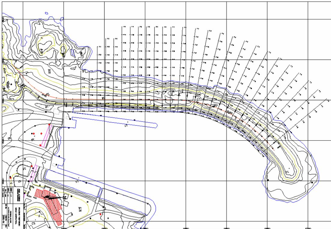
Figure 2 Plan of survey lines and elevation isolines in the 2005 survey.
