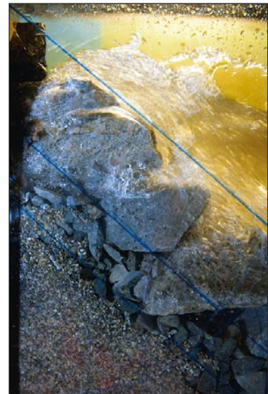
Breakwater model tests Photo: NTNU Info
