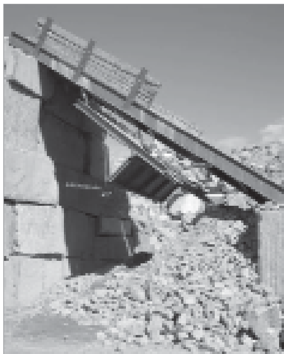
Figure 3.84 Large static bar for production of different grading sizes (courtesy S Dupray)
