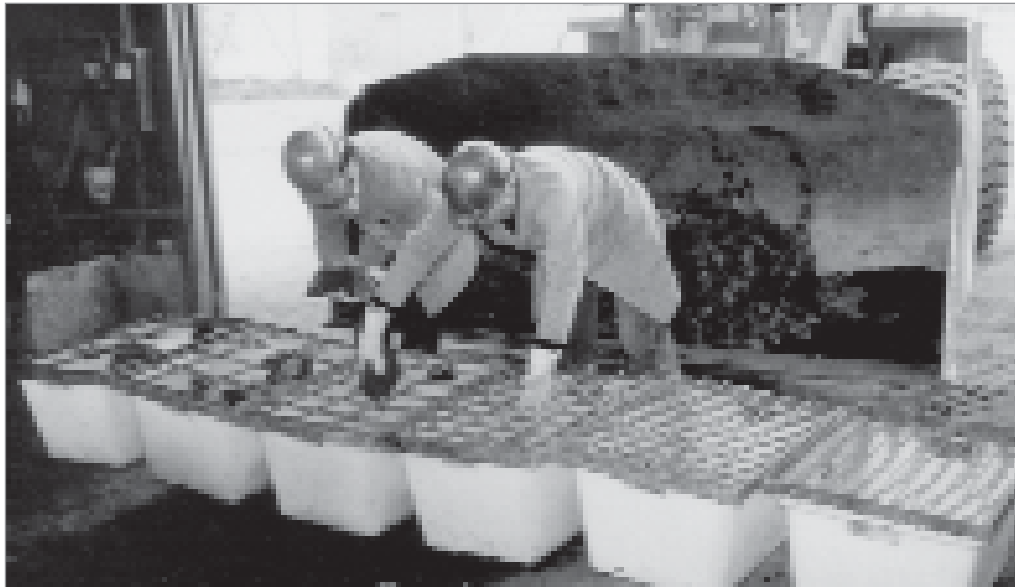
Figure 3.40 Steel rod sieves in use for determination of size distribution of a coarse grading (courtesy G Laan)
