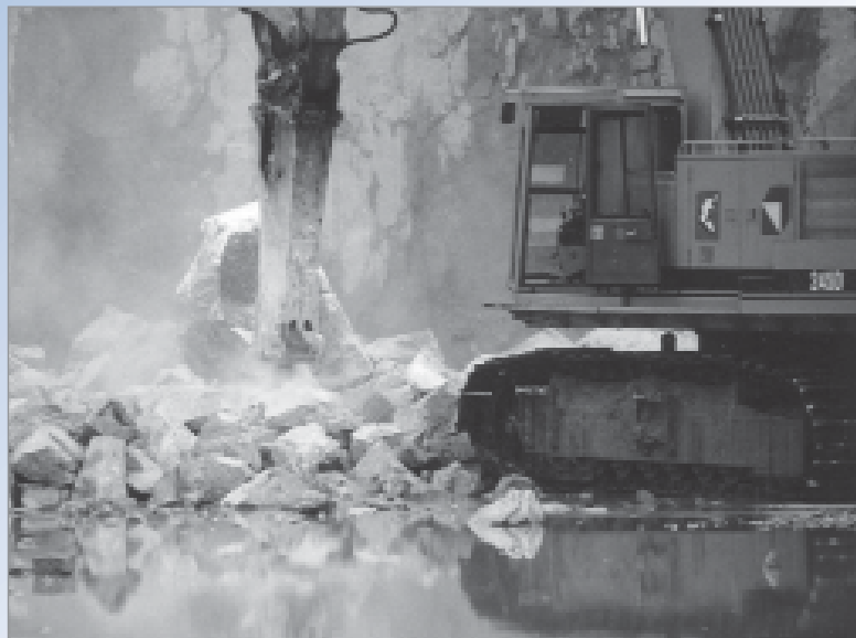
Figure 3.76 Hydraulic excavator with 3.5 t hydraulic hammer (courtesy J van Meulen)
