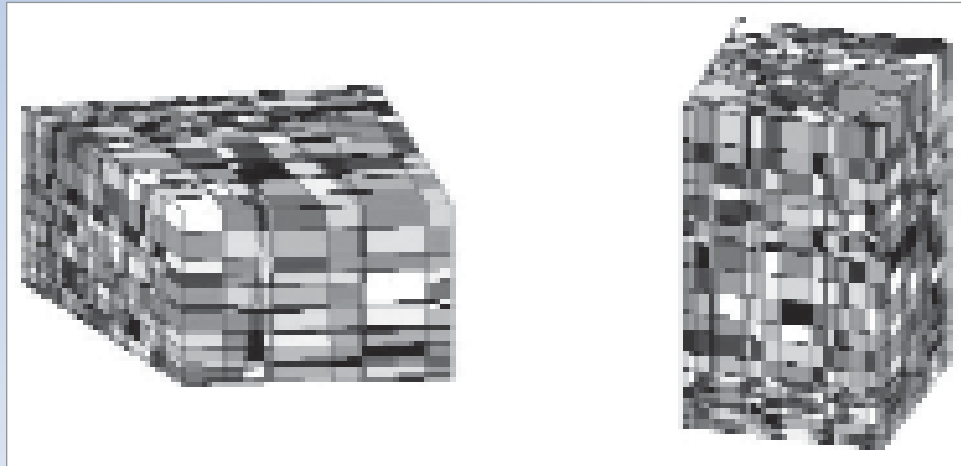
Figure 3.60 Computational dissection of rock masses – left: from Zone B (2100 m 3 ); right: Zone D (975 m 3 ) – using discontinuity location and orientation data from three perpendicular scanline segments
