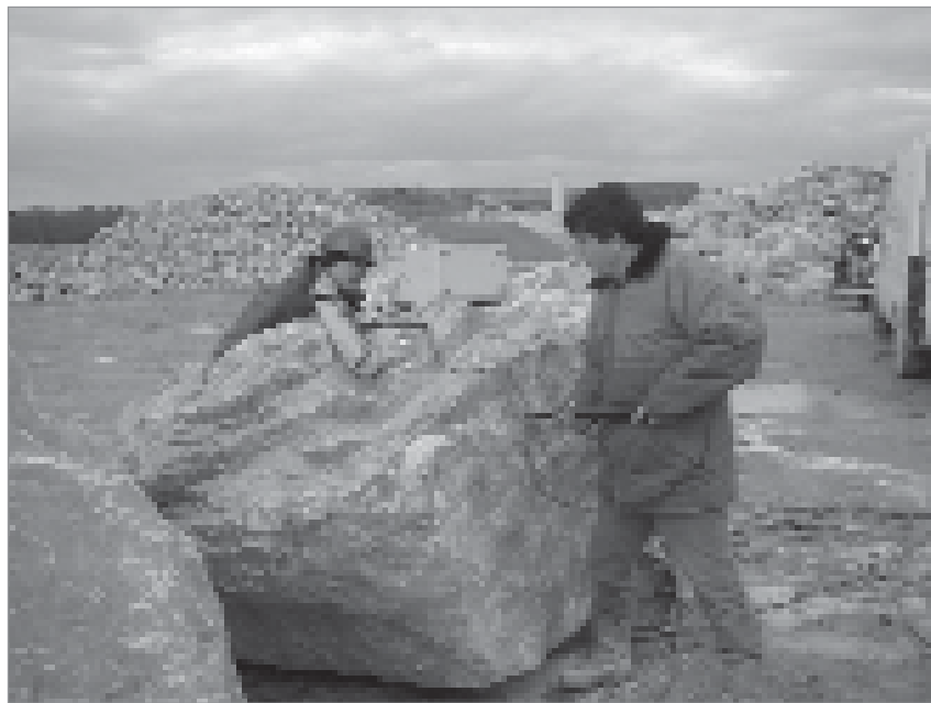
Figure 3.88 Testing of integrity of heavy armourstone using a sonic velocity concrete tester (courtesy T Wojnowski). Note the different stockpiles in the background
