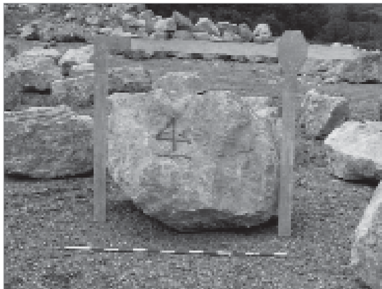
Figure 3.82 Use of a calliper for LT testing and quality control of blocks for the determination of strategically positioned “visual comparison blocks” used for control of shape (courtesy A Moiset)
