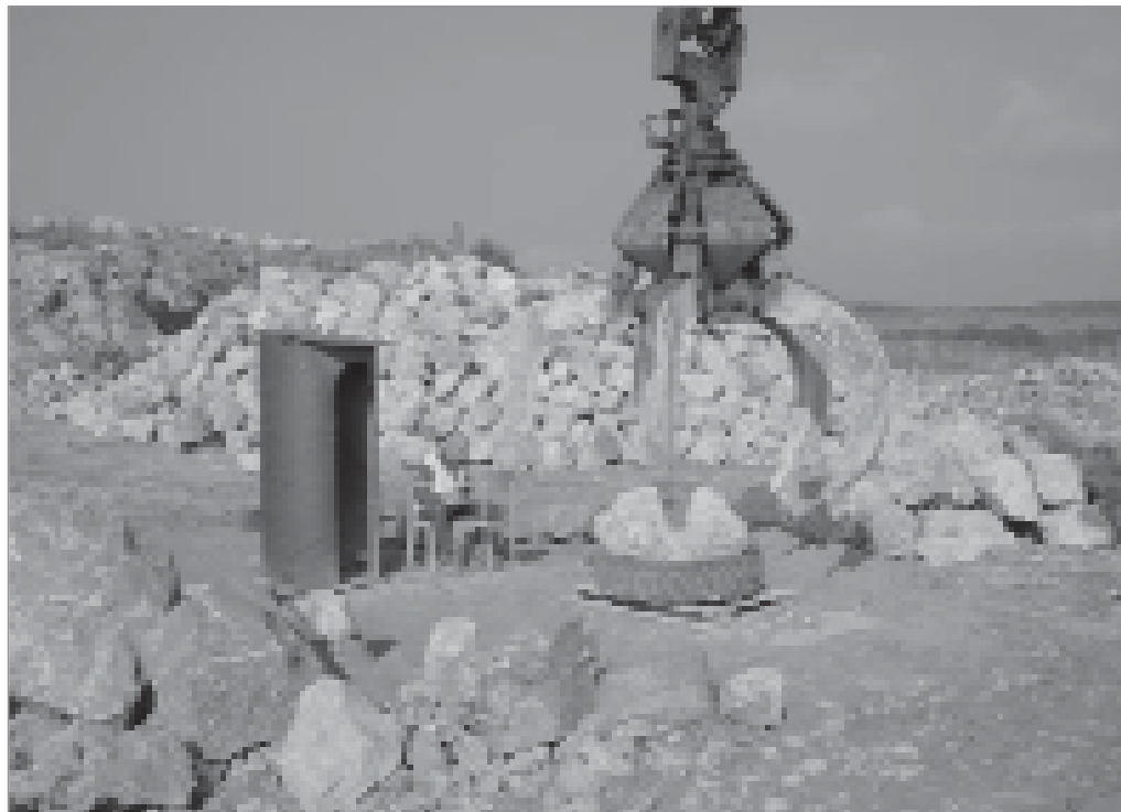
Figure 3.81 Control testing of mass distributions of a 300–1000 kg standard grading during production using weighbeams (courtesy A Moiset). This set-up enabled 140 stones to be weighed per hour
