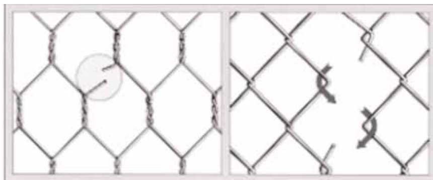
Figure 3.104 The advantage of double-twisted over chain link mesh
