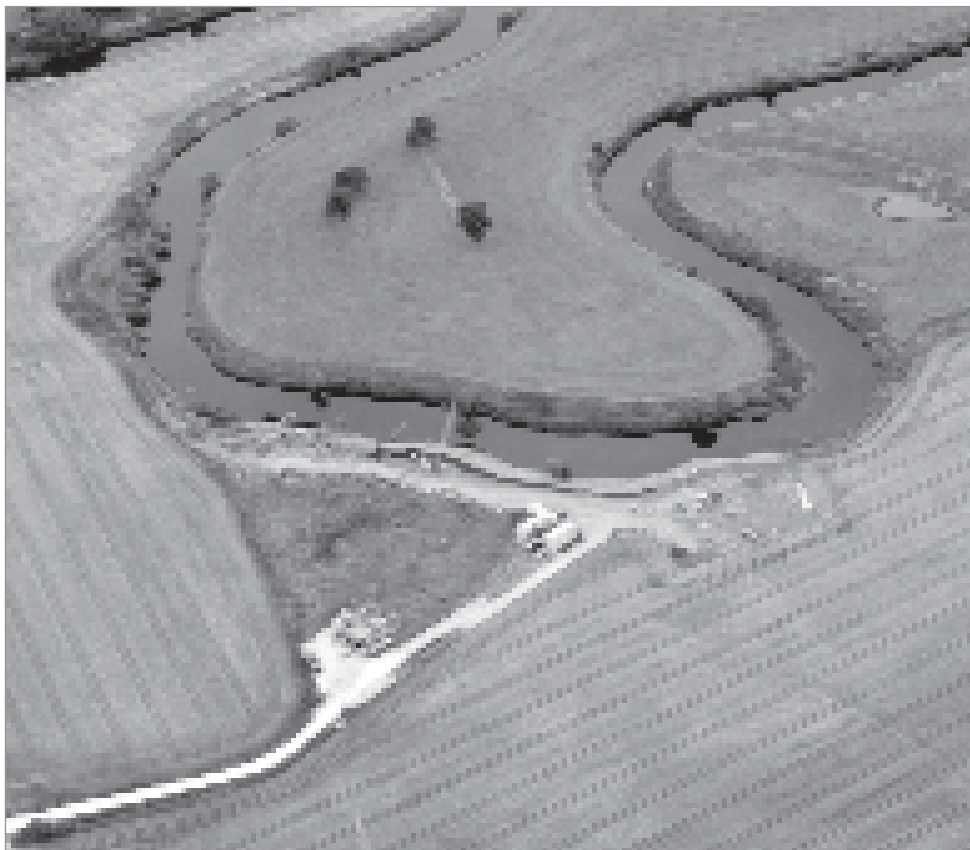
Figure 8.44 Aerial photograph of an armourstone revetment required to stop erosion of the bank exposing contaminated soils. Note: The alignment in Figure 8.44 follows the line of the bank and ties into more stable bank at either end. The retention of shrubs in the riverbank (courtesy Mott MacDonald)
