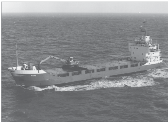
Figure 9.39 Self-loading and discharging vessel MV Mari (courtesy Sillanpää)
