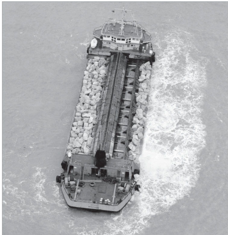
Figure 9.30 Dynamic positioning of side stone-dumping vessel Cetus with bow and stern thrusters (courtesy Royal Boskalis Westminster)
