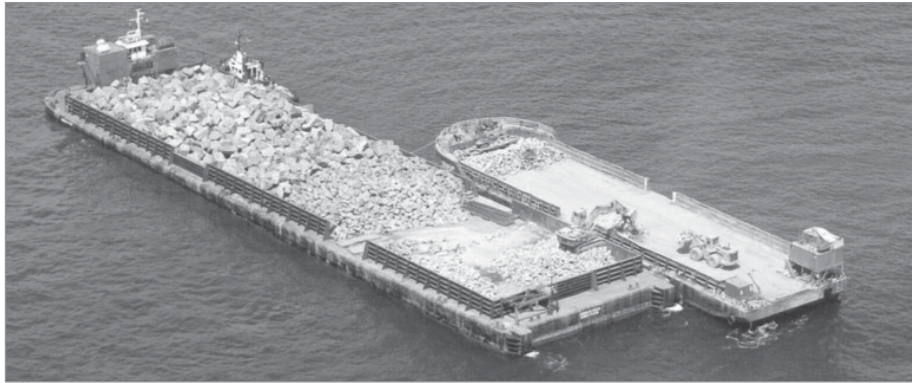
Figure 9.38 Flat-top barge carrying 20 000 t of armourstone (courtesy Stema Shipping (UK) Ltd)
