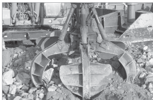
(a) Cactus/orange-peel/closed-tine grab (often termed a grapple in scrap iron works)
